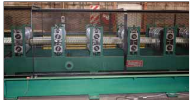
Above and below: The machine that produces Tray-dec's new products, which were designed in-house, was designed and built by Hayes International in Rotorua.
